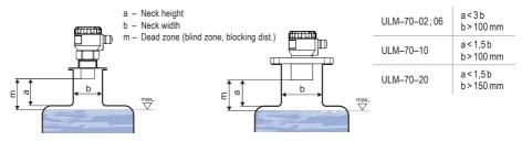
Fig. 4: Possible installation of the installation neck
