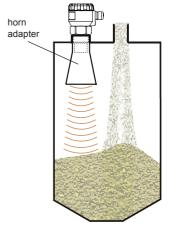
Fig. 8: Level meter installation in silo or hopper
