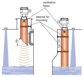
Obr. 12a: Short guide tube installation
