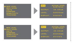
ACTUAL LEVEL: Actual distance to level OUTPUT: current 4 mA / 20 mA LEVEL: Definition of the min / max level DISPLAY: The value showed on the display
