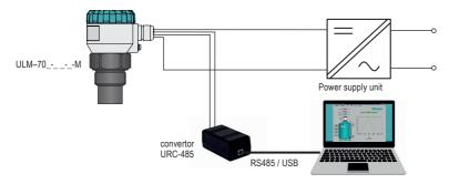
Obr. 23: Typical hardware configuration with Modbus®
