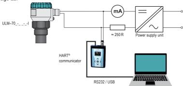
Obr. 22: Typical hardware configuration with HART
